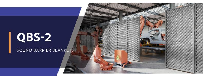
The barrier septum configuration offers the benefits of both sound absorbers and noise barriers. The **QBS-2** blanket by NetWell consists of a non-reinforced 1 lb-psf loaded vinyl noise barrier sandwiched between two layers of quilted acoustical fiberglass, each faced with a vinyl-coated-fiberglass-cloth. One side has a 2" thick quilted layer to face the noise source for maximum sound absorption. The other side has a 1" thick quilted layer to act as a decoupler against a wall.
