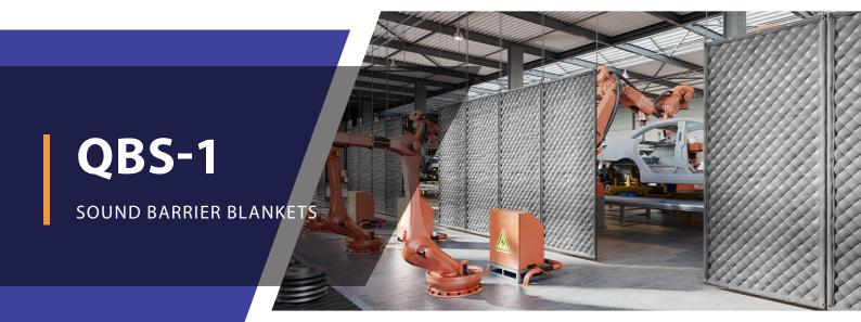
The barrier septum configuration offers the benefits of both sound absorbers and noise barriers. The **QBS-1** blanket by NetWell consists of a non-reinforced 1 lb-psf loaded vinyl noise barrier sandwiched between two layers of 1" thick acoustical fiberglass sound absorbers, each quilted with a vinyl-coated-fiberglass-cloth facing.
